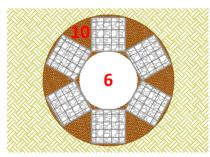
Upper tier of gabions rotated by 30° (lower tier shaded)
